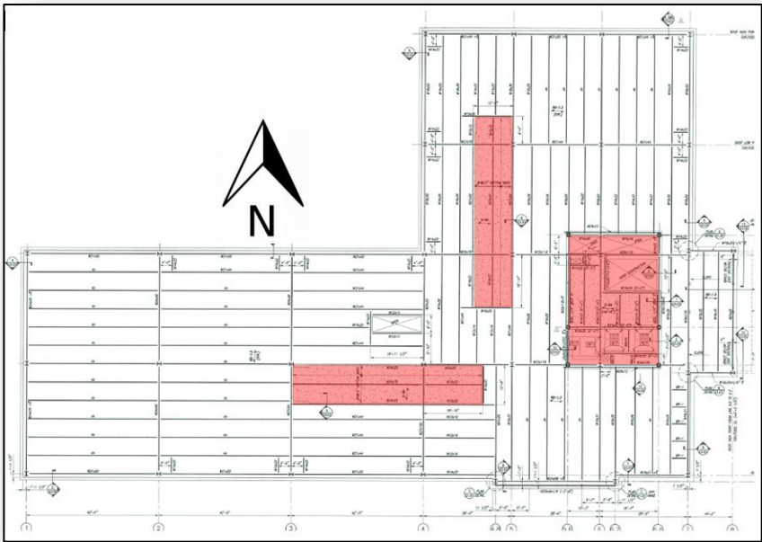
Figure 15: Roof Framing Plan – S1.07
